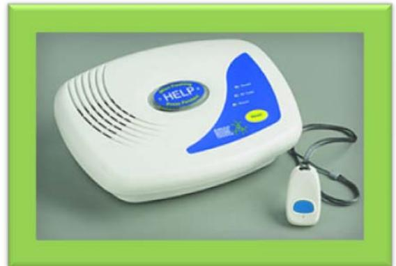
One successful application is the Personal Emergency Response System (PERS)<sup>1</sup>. A Personal Emergency Response System is a system which allows individuals, including older adults, to summon help during an emergency. Although PERS vary in specifications, the most common configuration has three components:
